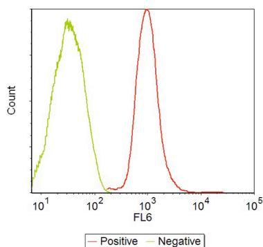
**Figure 3.** A typical flow cytometry based protein detection assay result using Zepto™ Ultra Carboxyl Microspheres. The figure shows a histogram of a negative sample (green) and a positive sample (red) containing the target of interest. Note the increase in fluorescence of the positive sample due to binding of the fluorophore-labeled reporter antibody.
