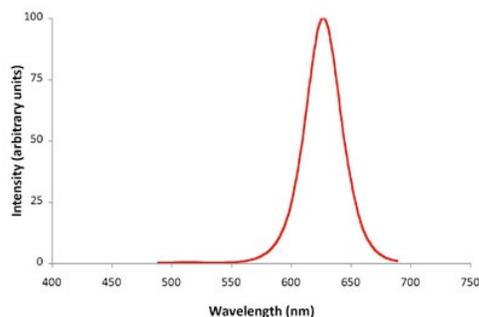
**Figure 1.** Emission spectrum of Zepto™ Ultra Orange Carboxyl Microspheres.
